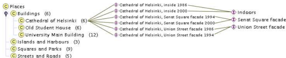
Figure 19: On the left side of the classes that have subclasses is a ball-like symbol with a line pointing either down or right. Right-position indicates that the subclass-structure is hidden, and down-position indicates it is revealed.
